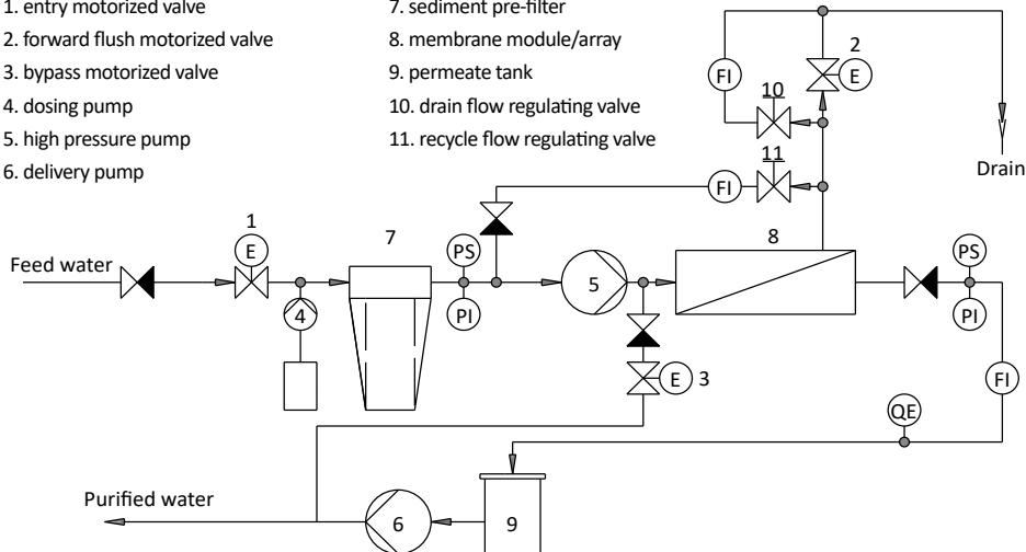
Figure 2. Reverse osmosis system with permeate rinsing
