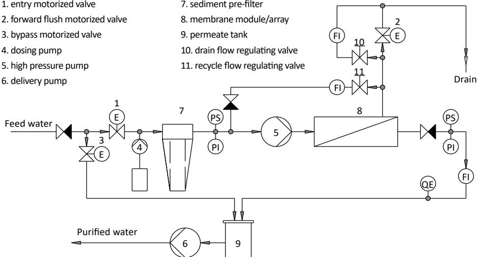
Figure 1. Reverse osmosis system with raw water blending
